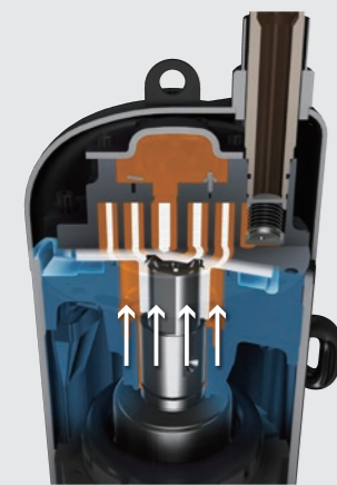
The force pressing the orbiting scroll decreases during low-load operation.
